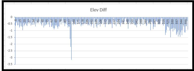
Based on the 95% Confidence (Accuracy<sub>z</sub>) value of 1.25', Fig 2 indicates that this data would support 2' contour intervals.
