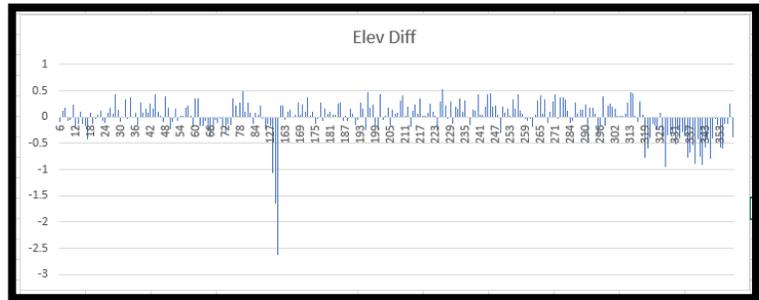
Based on the 95% Confidence (Accuracy<sub>z</sub>) value of 0.66', Fig 2 indicates that this data would nearly support 1' contour intervals.
