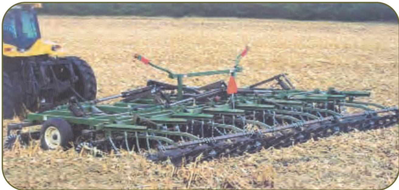
**FOR RUSLE2 CALCULATIONS THIS IS THREE OPERATIONS—COULTER CADDY AND A ROLLING CULTIVATOR. NOTE: THIS TURBO-TILL HAS A ROLLING BASKET INSTEAD OF THE COIL TINE HARROW.**
