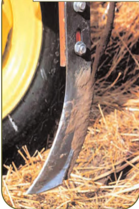
IN THE MIDWEST ANHYDROUS AMMONIA COMPRISES THE MAJORITY OF COMMERCIAL NITROGEN APPLICATION. ANHYDROUS AMMONIA MUST BE INJECTED INTO THE SOIL. THIS IS COMMONLY DONE WITH NARROW KNIVES ATTACHED TO A TOOL BAR PULLED BY A TRACTOR. PRECISE APPLICATION IS IMPORTANT FROM ECONOMIC AND ENVIRONMENTAL PERSPECTIVES.
