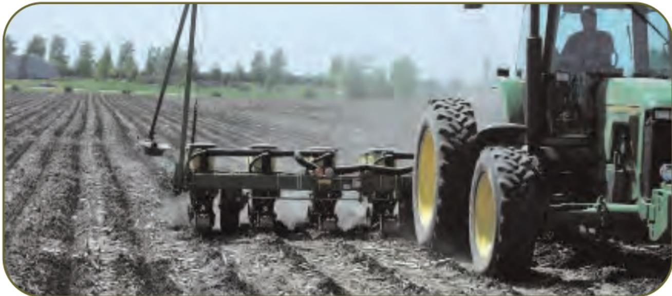
**SEEDBED PREPARATION IS COMPLETED IN A NARROW BAND NO MORE THAN 1/3 OF THE ROW WIDTH. IT MAY BE COMPLETED IN THE FALL WITH THE APPLICATION OF NUTRIENT OR AT PLANTING TIME. CROP RESIDUE AND SOIL CONSOLIDATION IS LEFT UNDISTURBED BETWEEN THE SEEDBED AREAS.**
