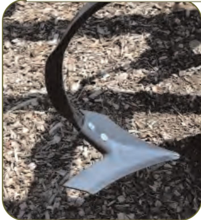
FIELD CULTIVATORS EQUIPPED WITH SWEEPS DO EXTENSIVE HORIZONTAL AND VERTICAL SOIL MIXING. SWEEPS ARE THE CHOICE FOR HERBICIDE INCORPORATION. SWEEPS BURY MORE RESIDUE THAN FIELD CULTIVATORS EQUIPPED WITH SPIKED POINTS.
