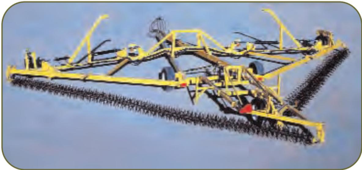
THE PHILLIPS™ ROTARY HARROW WORKS IN THE TOP INCH OR SO TO PREPARE SEEDBEDS. IT REDISTRIBUTES RESIDUE AND LEVELS THE GROUND. (\*DEPENDING UPON THE TYPE OF RESIDUE PRESENT, USE HARROW ROTARY FOR HEAVY, NONFRAGILE RESIDUE SUCH AS CORN AND HARROW ROTARY LIGHT FLUFF FRAGILE FOR LIGHT RESIDUE SUCH AS SOYBEANS.)
