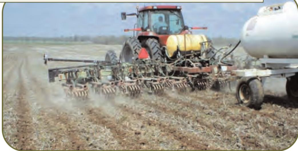
STRIP TILLAGE COMBINES THE BENEFITS OF NO-TILL AND FULL-WIDTH TILLAGE, BUT TILLAGE IS CONFINED TO 6- TO 8-INCH STRIPS INTO WHICH DRY FERTILIZER AND/OR ANHYDROUS AMMONIA CAN BE PLACED. LOOSENEED SOIL IN THE STRIPS CREATES A RIDGE OR BERM 3 TO 4 INCHES HIGH, WHICH SETTLES DOWN TO 1 TO 2 INCHES BY SPRING PLANTING. CROP RESIDUE IN ROW MIDDLES IS LEFT UNDISTURBED.
