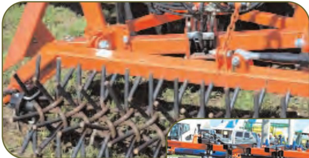
THE PHOENIX® HARROW IS USED TO MIX THE TOP INCH OF SOIL SURFACE TO INCORPORATE HERBICIDES AND LEVEL THE GROUND. THE ANGLE MAY BE ADJUSTED FROM 20 TO 45 DEGREES.
