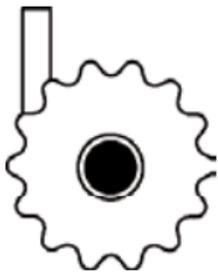
NOTCHED DISKS ARE VERY SIMILAR TO THE CONCAVE DISK AND DEPENDS UPON THE SIZE AND DEPTH OF TILLAGE AS TO HOW MUCH SOIL DISTURBANCE IS DONE.
