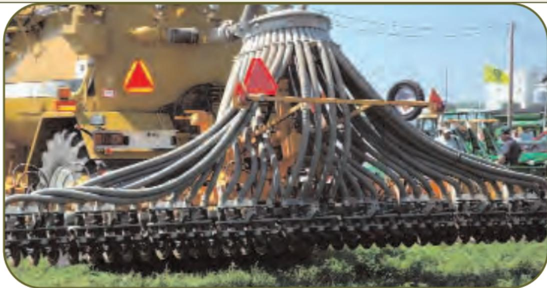
TANK TYPE LIQUID MANURE INJECTOR WITH LOW DISTURBANCE COULTERS. HOWEVER, BECAUSE 15 INCH ROWS ARE USED HERE, THIS METHOD DISTURBS TWICE AS MUCH SOIL SURFACE AS WHEN 30 INCH ROWS ARE USED. AS A RESULT RUSLE2 SOIL LOSS CALCULATIONS WILL BE HIGHER WITH 15 INCH VERSUS 30 INCH UNITS.
