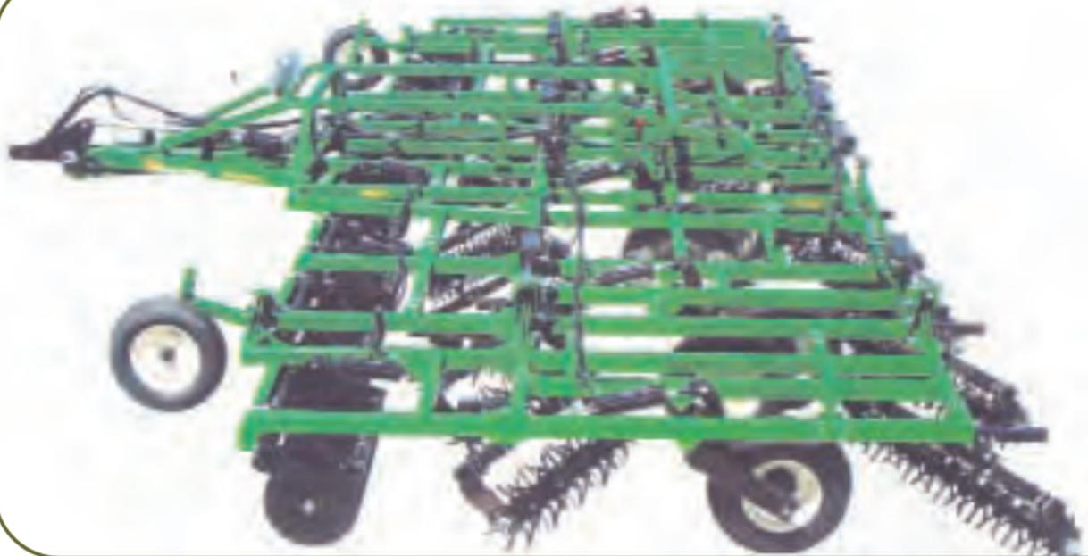
**FOR RUSLE2 CALCULATIONS THIS TILLAGE TOOL IS THREE OPERATIONS—ONE COULTER CADDY AND TWO PHILLIPS™ HARROWS.**
