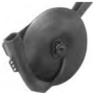
SINGLE DISK OPENERS ARE USED TO CUT THE SURFACE RESIDUE.
