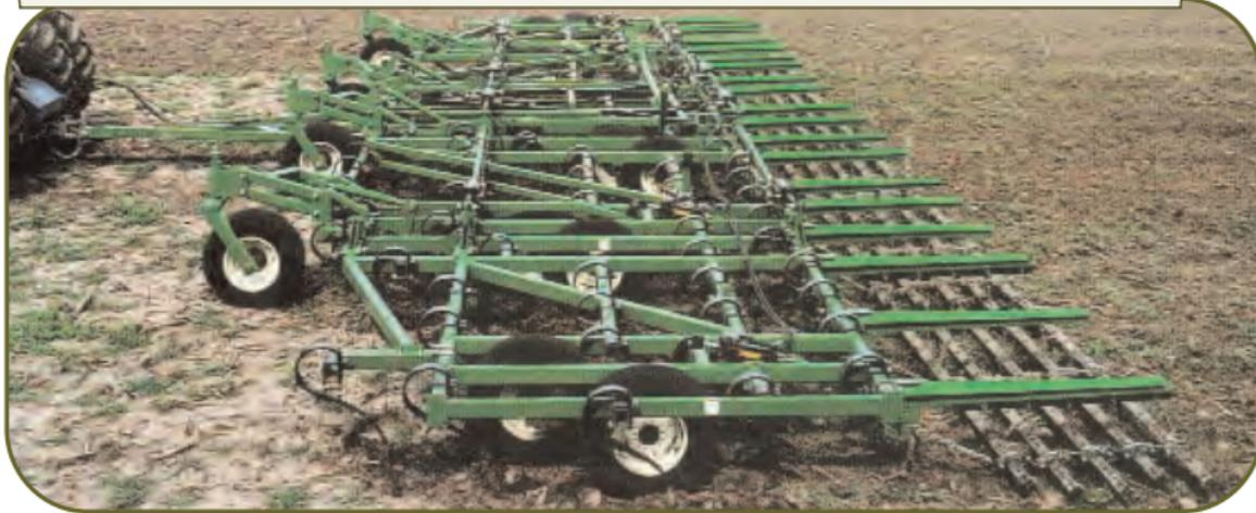
A FIELD CULTIVATOR IS DESIGNED FOR LIGHT TILLAGE AND FIELD FINISHING. USUALLY THEY ARE USED FOR SECONDARY TILLAGE AND FOR INCORPORATING HERBICIDES. SPIKED POINT FIELD CULTIVATORS DO LITTLE SOIL MIXING AND LEAVE MORE RESIDUE ON THE SURFACE.
