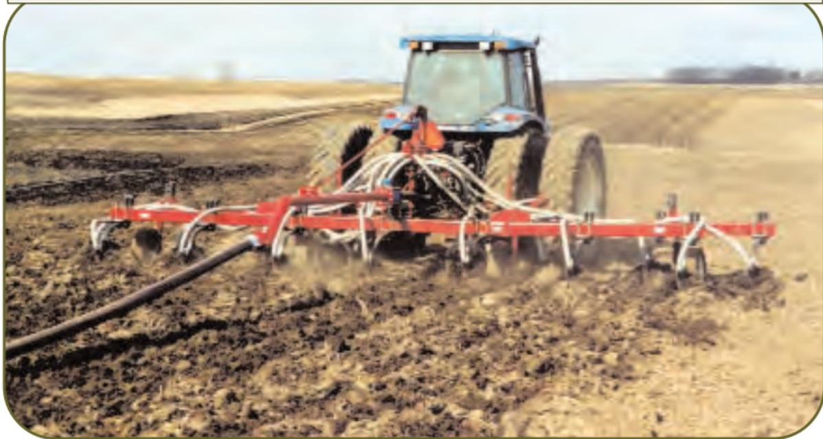
WHEN USING AN UMBILICAL CORD MANURE INJECTION SYSTEM ON 30 INCH SPACING IN BEAN STUBBLE, THE TYPE OF INJECTOR SYSTEM WILL DETERMINE THE AMOUNT OF RESIDUE AND SOIL DISTURBANCE.
