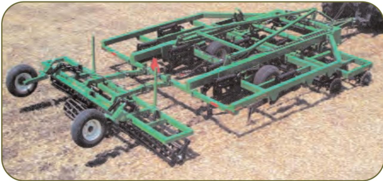
**VERTI-TILL IS A COULTER/SUBSOILER DESIGNED TO CUT AND SIZE RESIDUE, AS WELL AS DEEP RIP HORIZONTAL DENSITY LAYERS IN ONE PASS. FOR RUSLE2 CALCULATIONS THIS IS THREE OPERATIONS—COULTER CADDY WITH SUBSOILER AND ROLLING CULTIVATOR.**
