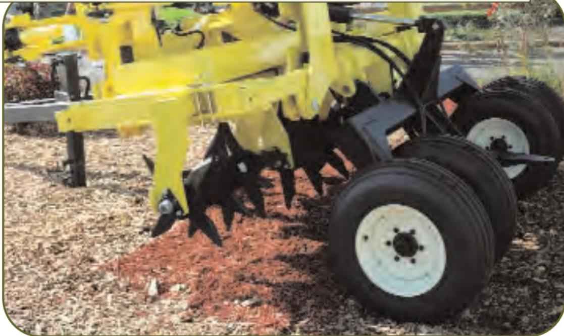
**WHILE MAINTAINING SURFACE RESIDUE, SHATTERTINES CRACK AND SHATTER COMPACTED SOIL 8 INCHES TO OPEN NEW CHANNELS FOR AIR AND WATER.**
