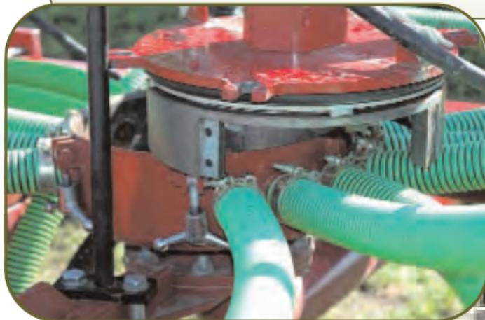
PICTURED ABOVE IS A DISASSEMBLED MANURE DISTRIBUTION BOX WHICH USES HIGH SPEED ROTATING KNIVES TO CUT MANURE CHUNKS INTO A NON-CLOGGING SIZE. TO THE RIGHT IS A CLOSE UP OF THE DISKS AND INJECTION BLADES.
