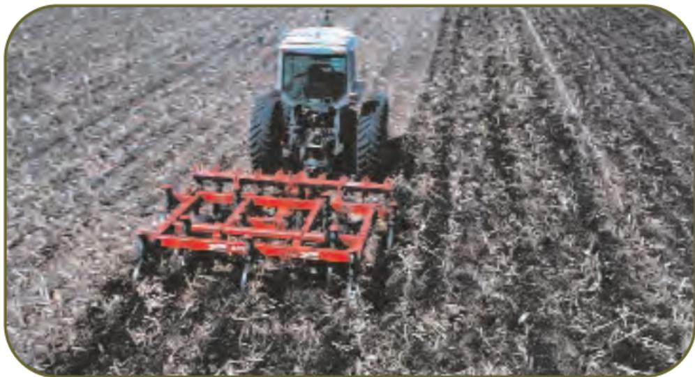
**MULCH-TILL - THE SOIL IS DISTURBED THE FULL WIDTH PRIOR TO PLANTING. TILLAGE TOOLS SUCH AS CHISELS, FIELD CULTIVATORS OR DISKS ARE USED FULL WIDTH. WEED CONTROL IS ACCOMPLISHED WITH HERBICIDES AND/OR CULTIVATION.**
