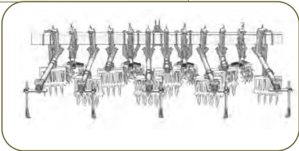
**A ROLLING CULTIVATOR USES TWO SPIDER GANGS ON EACH ROW ASSEMBLY. IT OPERATES IN HEAVY RESIDUE WITHOUT CLOGGING.**
