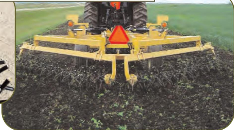
TINES DISTURB ONLY THE TOP INCH OR SO OF SOIL. IN GENERAL, THE GREATER A TOOL IS ANGLED OFF THE TOOL BAR, THE MORE THAT OPERATION WILL DISTURB THE SOIL. THE PHILLIPS™ HARROW IS PERMANENTLY SET AT A 45 DEGREE ANGLE. (DEPENDING ON THE TYPE OF RESIDUE PRESENT, USE HARROW ROTARY FOR HEAVY, NONFRAGILE RESIDUE SUCH AS CORN, AND HARROW ROTARY LIGHT FLUFF FRAGILE FOR LIGHT RESIDUE SUCH AS SOYBEANS.)
