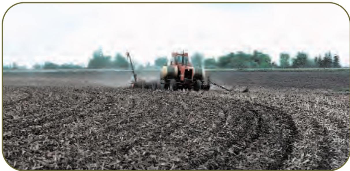
**MULCH-TILL PLANTING WILL LEAVE VARYING RESIDUE LEVELS AFTER PLANTING DEPENDING UPON THE NUMBER OF TILLAGE PASSES AND THE LEVEL OF SOIL DISTURBANCE.**
