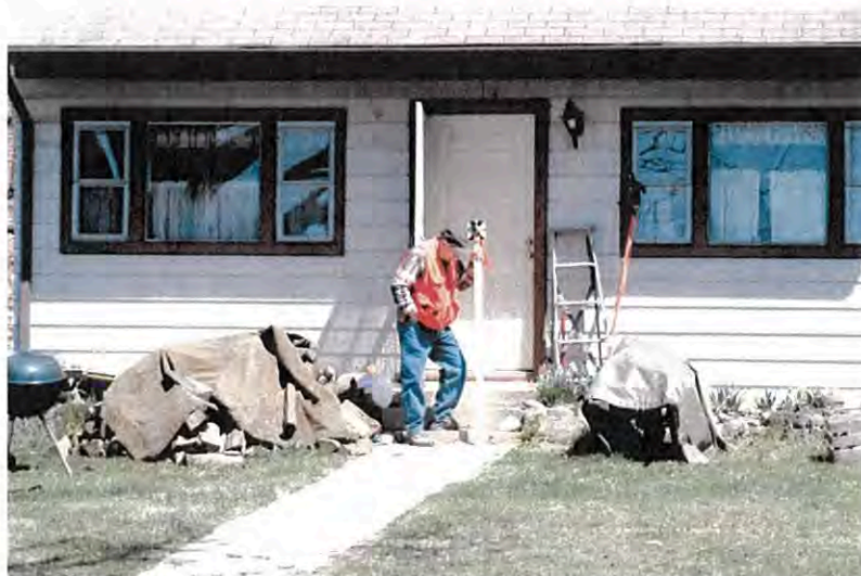
Figure 1 - Survey of first floor elevations and points of entry for all structures in the breach zone
