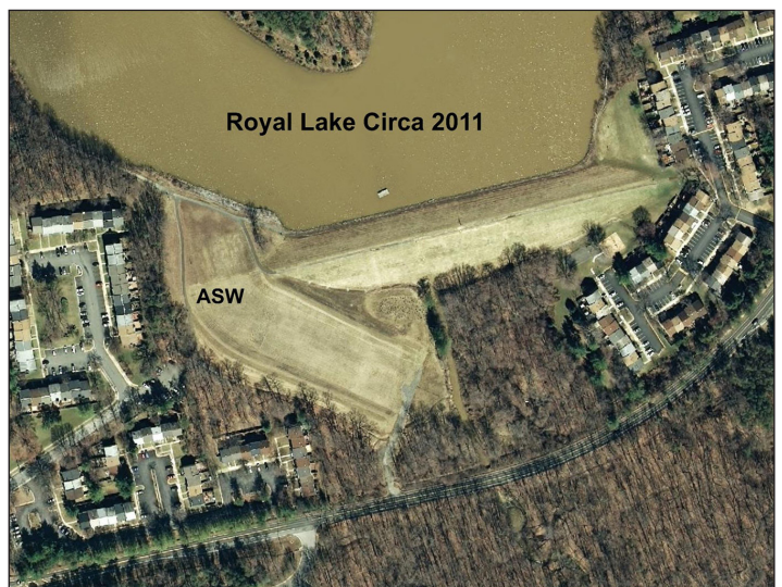
These before and after aerial photos of Royal Lake show how the auxiliary spillway was rerouted to move water away from the townhouses near the dam.
