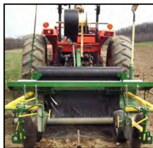
Figure 26. Tractor mounted mulch layer
