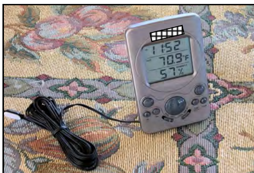
Figure 12. A relatively inexpensive indoor/outdoor hygrothermometer.
