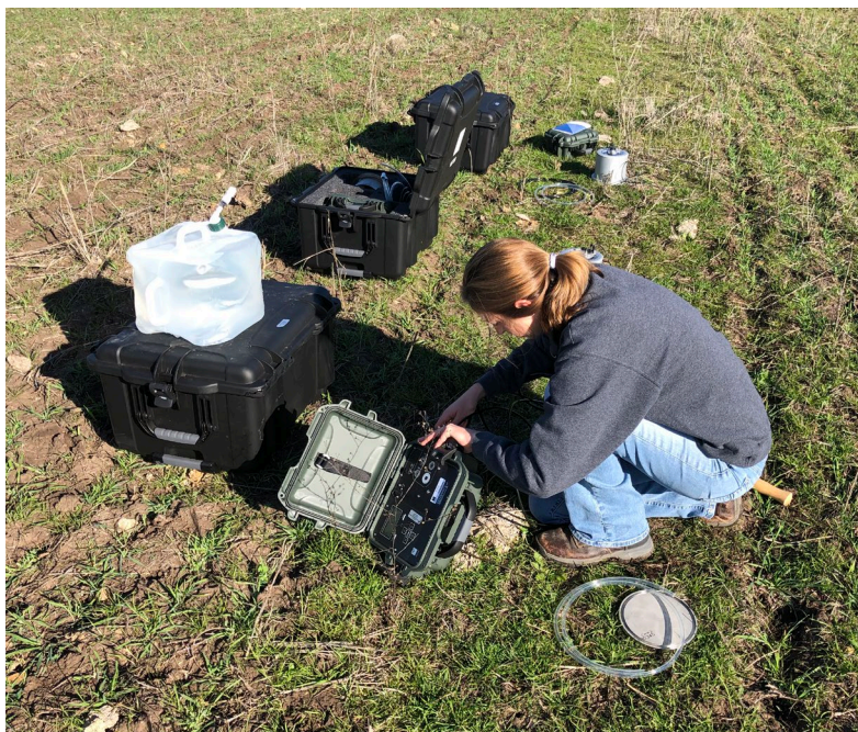
Ashley Anderson, soil scientist, sets up the SATURO Infiltrator to take the first field readings at the Roam Ranch.
