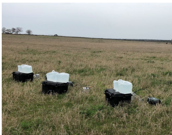
Infiltrators going through the cycles. Other than to check the progress and water tank levels, it does everything on its own.
