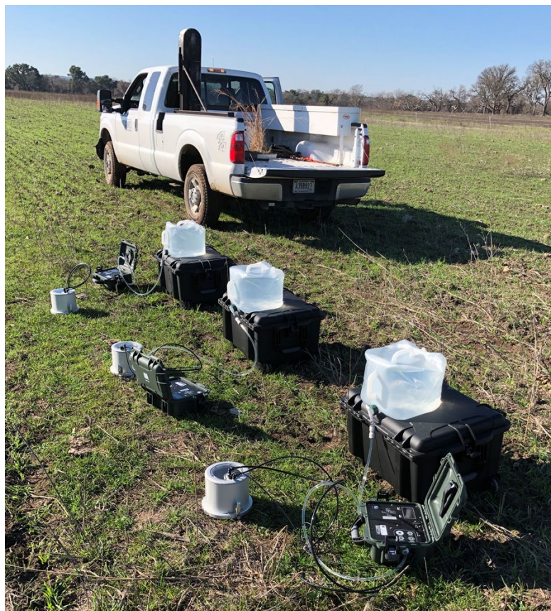
SATURO Infiltrometer site set-up.
