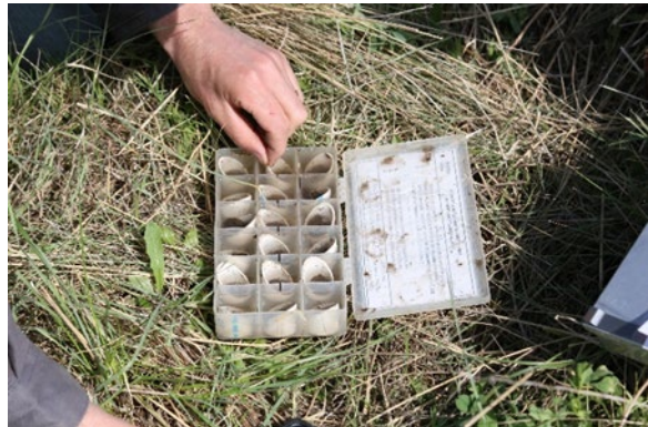
Slake test performed to measure the stability of the soil when exposed to rapid wetting.
