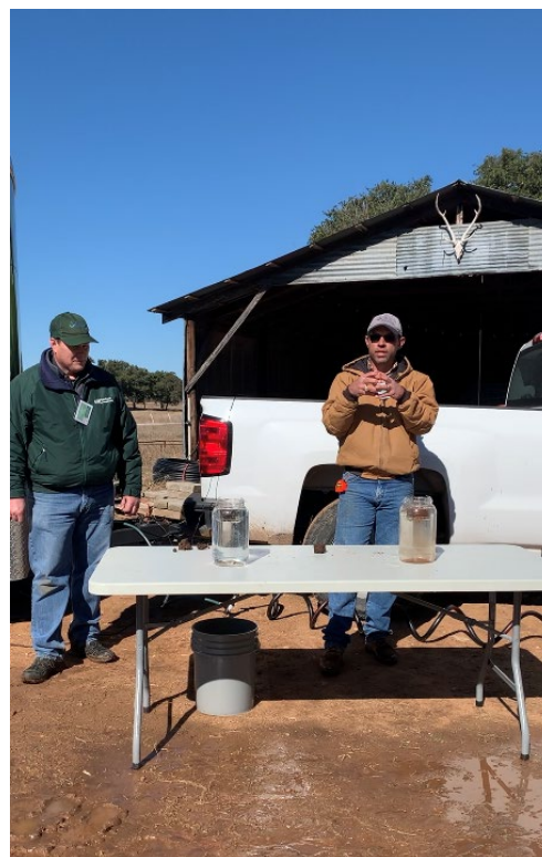
Dennis Brezina (left) and Travis Waiser (right) demonstrate how to set-up an “at-home” soil infiltration test.
