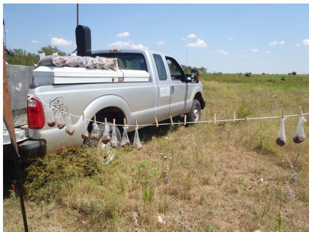
Soil bulk density clods dipped in liquid saran dry in the heat of an August day in Western Oklahoma. Bags of bulk soil samples taken from each horizon of the pedon can be seen on the truck toolbox.
