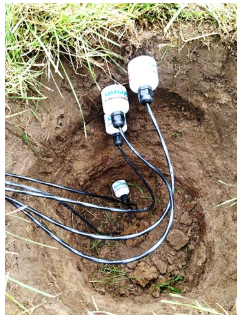
Figure 2. Soil sensors are placed at various depths to monitor soils moisture content and soil temperature.
