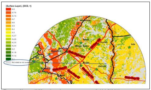
The area of interest (AOI) overlapped seven survey areas, of which 742,244 acres were identified with AASHTO surface errors "null" or "not rated". The staff will repair those errors to produce the intended results, as continued update and maintenance of the soils database is required to provide the best possible soils information to our customers.
