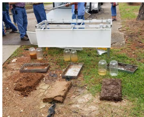
Soil sample boxes from the rainfall simulator are emptied for display, detailing the effects on soil erosion and stabilization.
