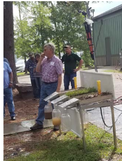
Mike Oliver, NRCS state forester, demonstrates the rainfall simulator.
