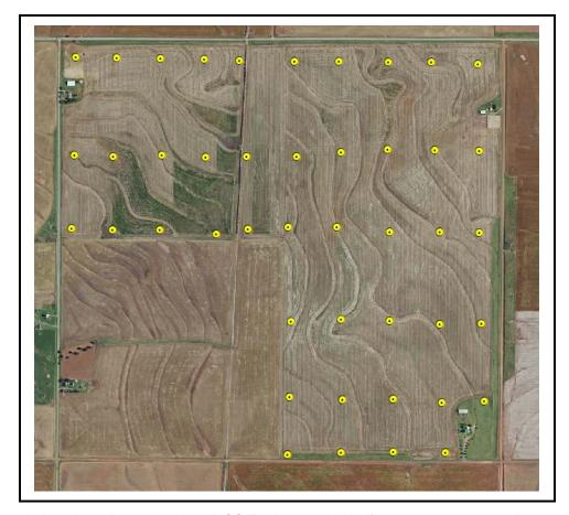
Sample locations determined by NRCS Engineers to identify water movement within the soils.
