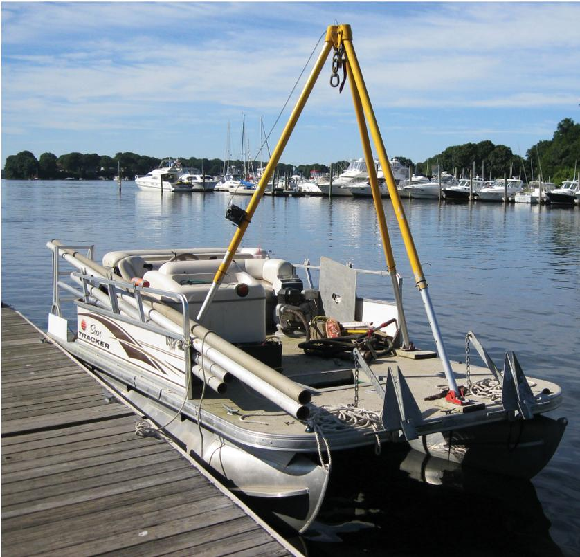
*A pontoon boat used for subaqueous soil sampling. The sampling is conducted through the moon-pool. A sealed core is strapped to the end of the chain fall. The chain fall is attached to the tripod, which is centered over the moon-pool.*
