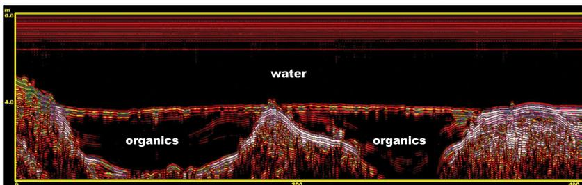
*GPR output for a freshwater lake with thick organic materials. Water, mineral soil materials, and organic soil materials are easy to identify from the output.*
