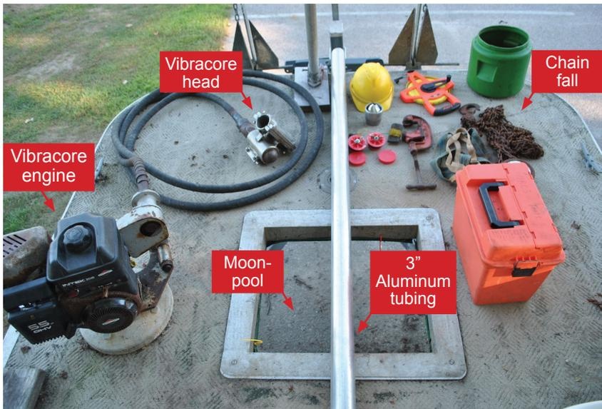
*Equipment for vibracore sampling. A vibracore sampler consists of an engine, cable, head, and core barrel. The engines are typically gasoline driven (sold as a device to keep concrete mixed so it does not set). The cable carries the vibrations to the head, which is attached to the core barrel with four bolts.*
