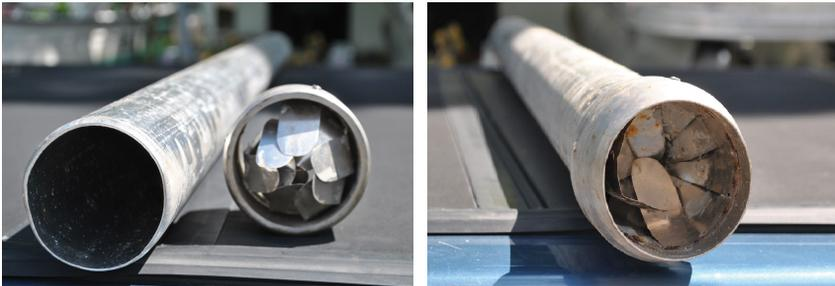
*A core barrel and core catcher. Left image—Core barrels used for vibracoring are typically 10 cm in diameter. The view of the sand catcher is from the perspective of the inside of the barrel. Right image—For sandy or loose materials, a core catcher may be attached to the bottom of the core barrel.*
